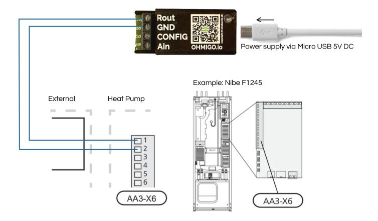
Connect GND and Rout on Ohm on WiFi to the inputs for the outdoor or room sensor on your device. Use a two-wire cable with at least 0.75 mm² conductors.
